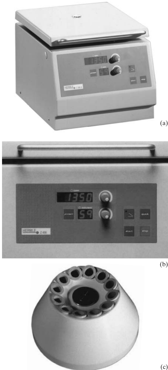
Plate 4.9 (a) Hermle Z 200 A, variable speed microprocessor controlled bench centrifuge.
