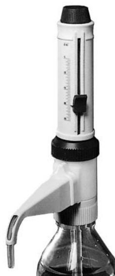
Plate 4.7 Labmax bottle top dispenser. Courtesy of Labnet International Inc.
