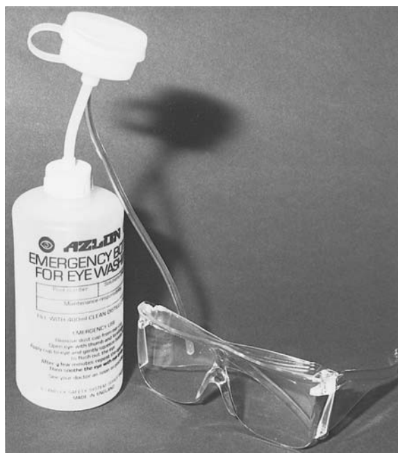
Plate 3.2 Left: 500ml emergency eye wash bottle. Squeezing the bottle gently sprays the eye. The waste liquid flows through a tube to the sink or collecting vessel. Instructions for use are printed in green on the bottle. Right: Protective eyeshields with closed in sides. The goggles are made from polycarbonate.
